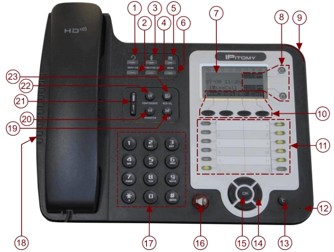
Figure 4 IPitomy IP320 Buttons and Hardware Definitions
